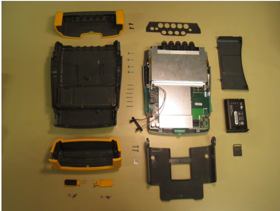
Fig. 6-1. Dismantling step 1 (bottom case removed)
