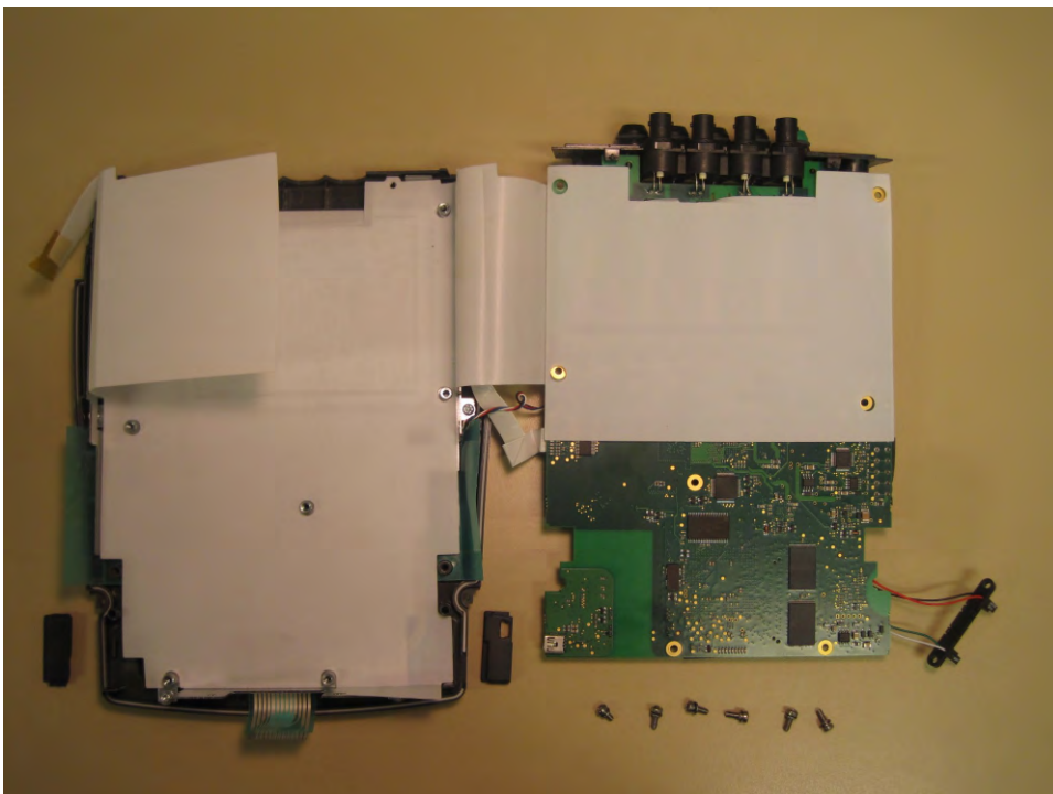
Fig. 6-3. Dismantling step 3 (PCA separated from chassis)
