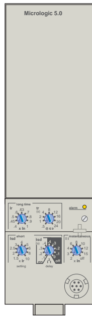
MicroLogic 3.0 and 5.0 Basic Trip Units
